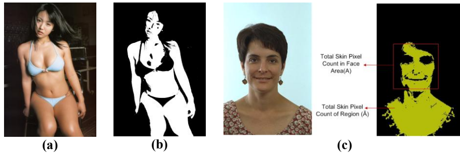
Fig. 2. (a) Input image, (b) its skin mask and (c) An example for close-up face elimination. Rectangular box indicates the face box given by the face detector.
