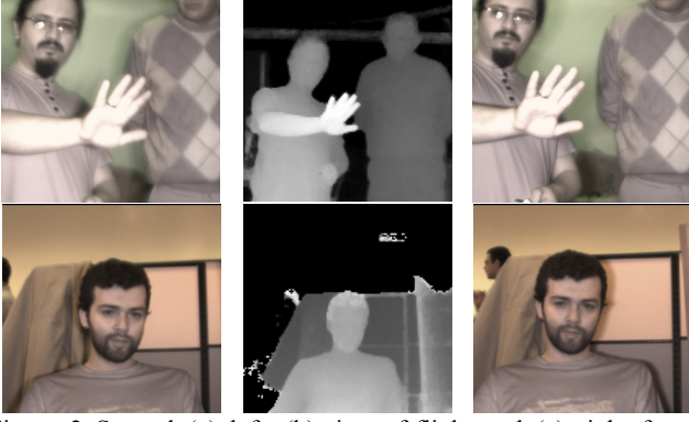
Figure 2 Several (a) left, (b) time-of-flight and (c) right frame groups as input.
